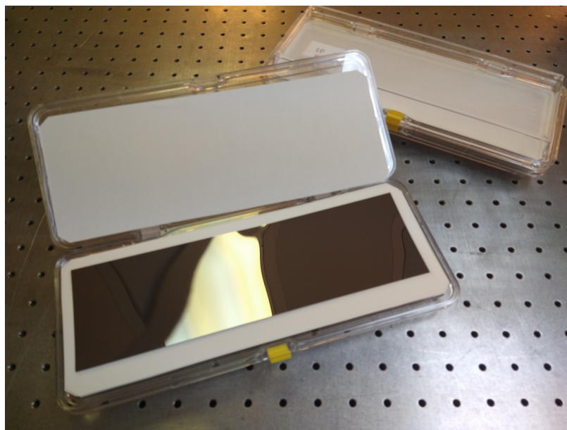
Blank silicon pieces of exact L0 and L1 sizes
