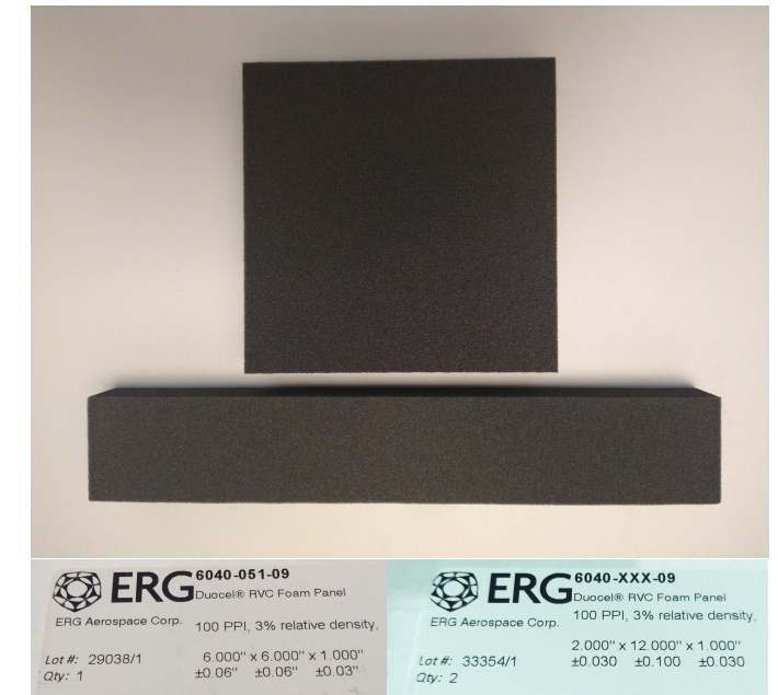
First samples of ERG Carbon RVC Duocel. Thanks to Nikki! Material sent to Genova for machining
