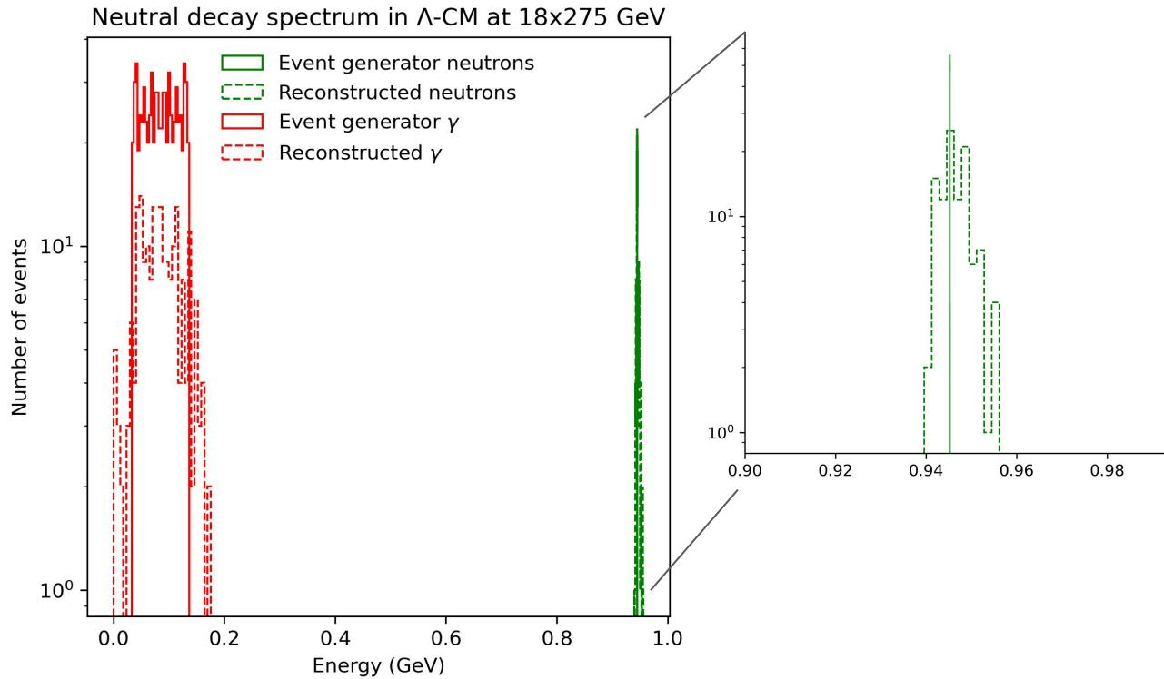
Conclusion: No neutron/ $\gamma$  mix up but resolution loss due to calorimeters stdev.
