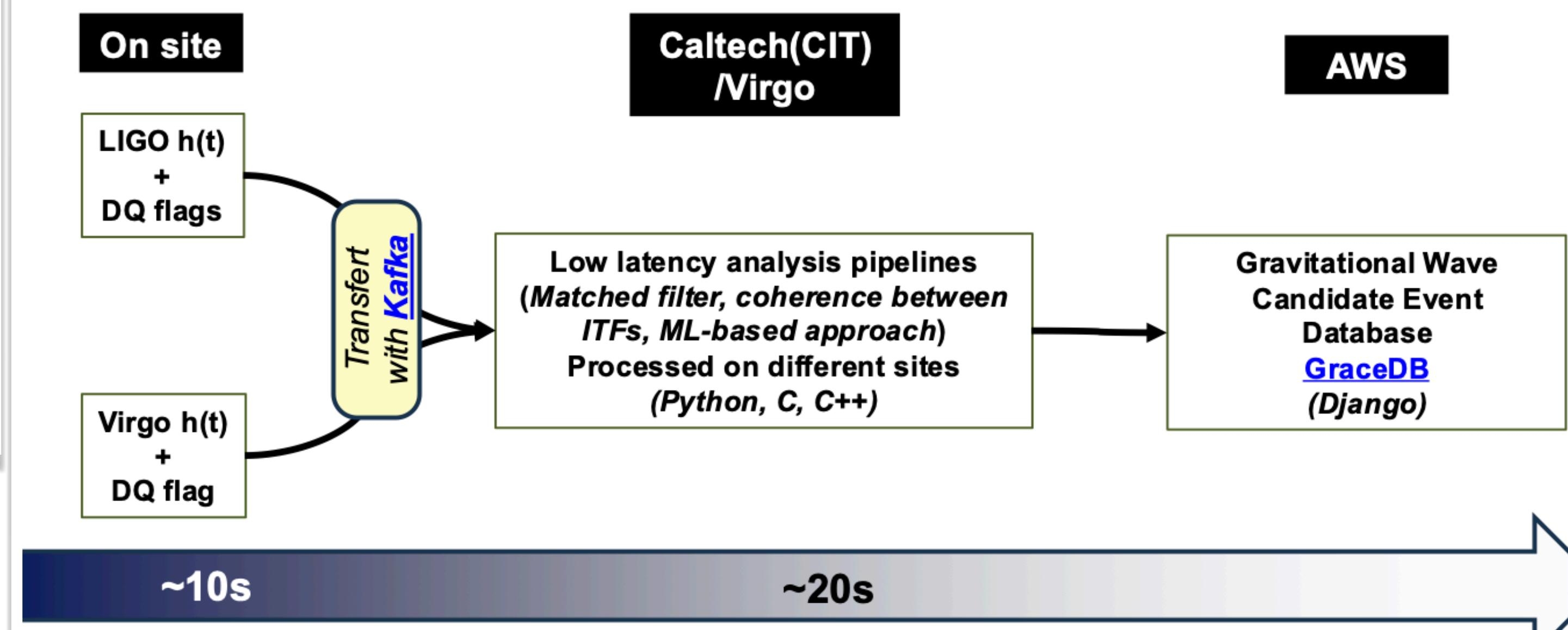
⇒ Less than 30s between an interesting event and the publication of the candidate on the DB. Low latency pipelines are highly parallelized in order to meet those requirements. CPU-based for the moment.
