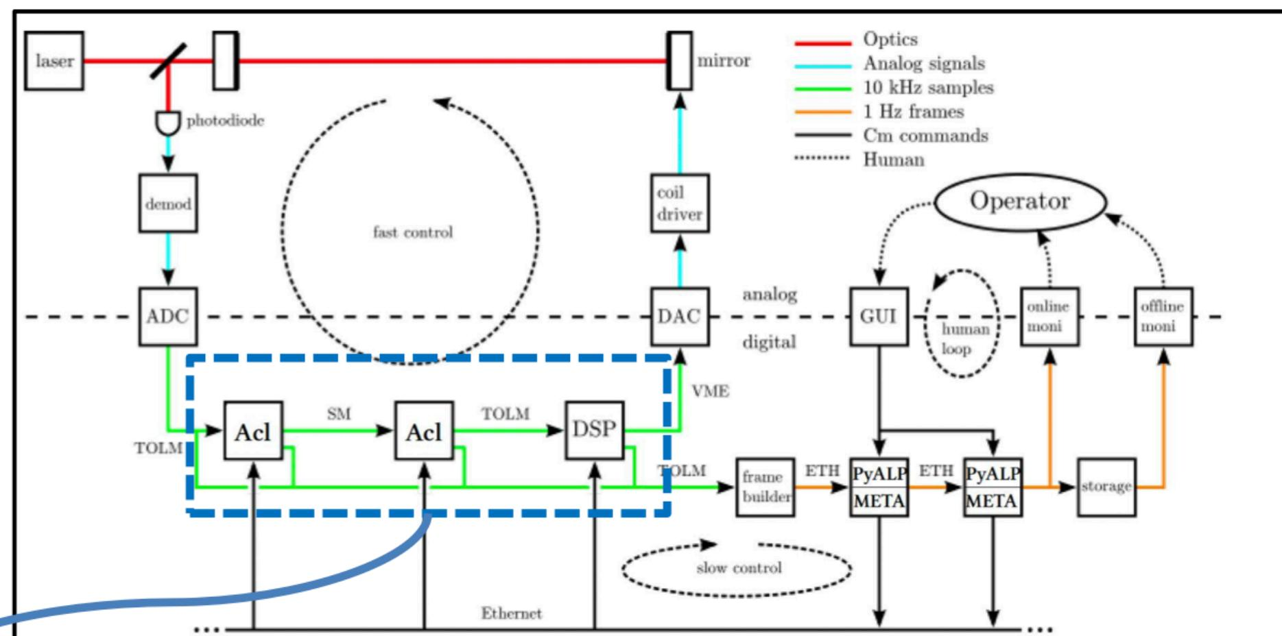
⇒ Real time control and calibration loops are handled either on RTPCs or on the DSP slices via dedicated custom low-level softwares: **ACL** for RTPCs (C code) and **DSPcode** for DSPs (Assembly code)
