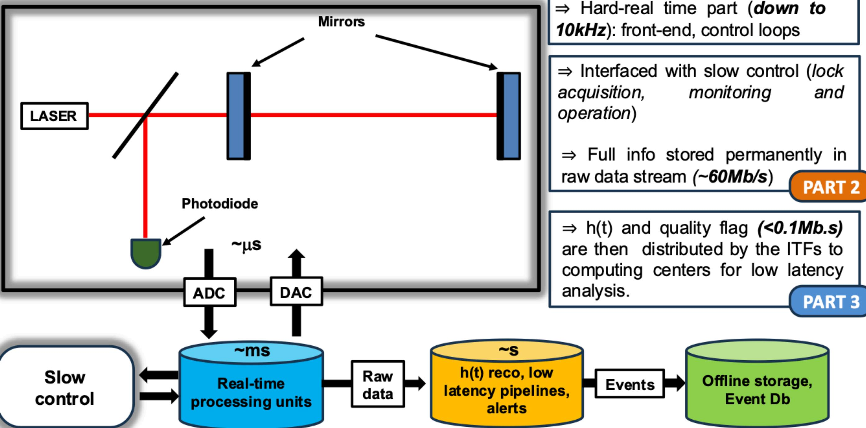
⇒ Virgo is triggerless by design. The deformation  $\Delta L/L = h(t)$  (aka *strain*) is continuously recorded as soon as the ITF is locked.
