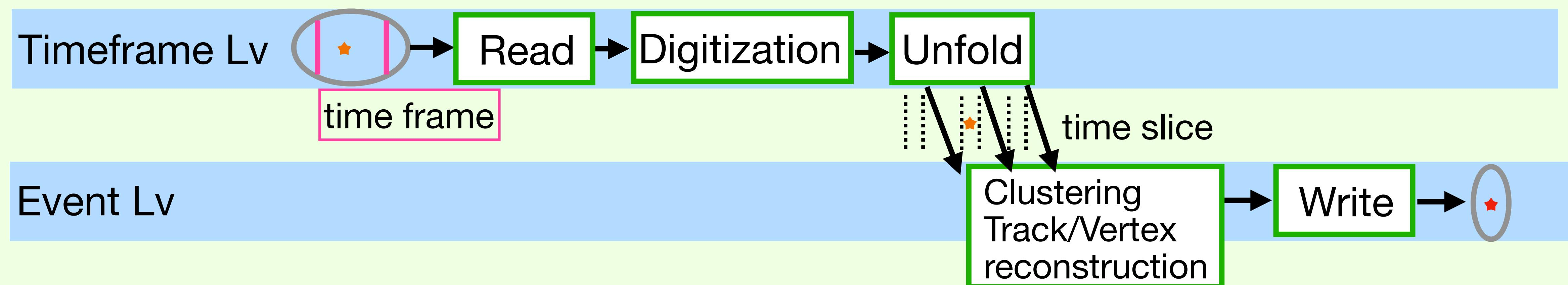
Splitting a single frame (time frame) into multiple frames (time slices) for parallel processing requires an **additional data stream**.
