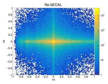
ePIC simulation, [25.08.0] Single neutron, p  $_{\rm MC}$  = 2.0 GeV/cFull detector Sum of bHCAL hits
