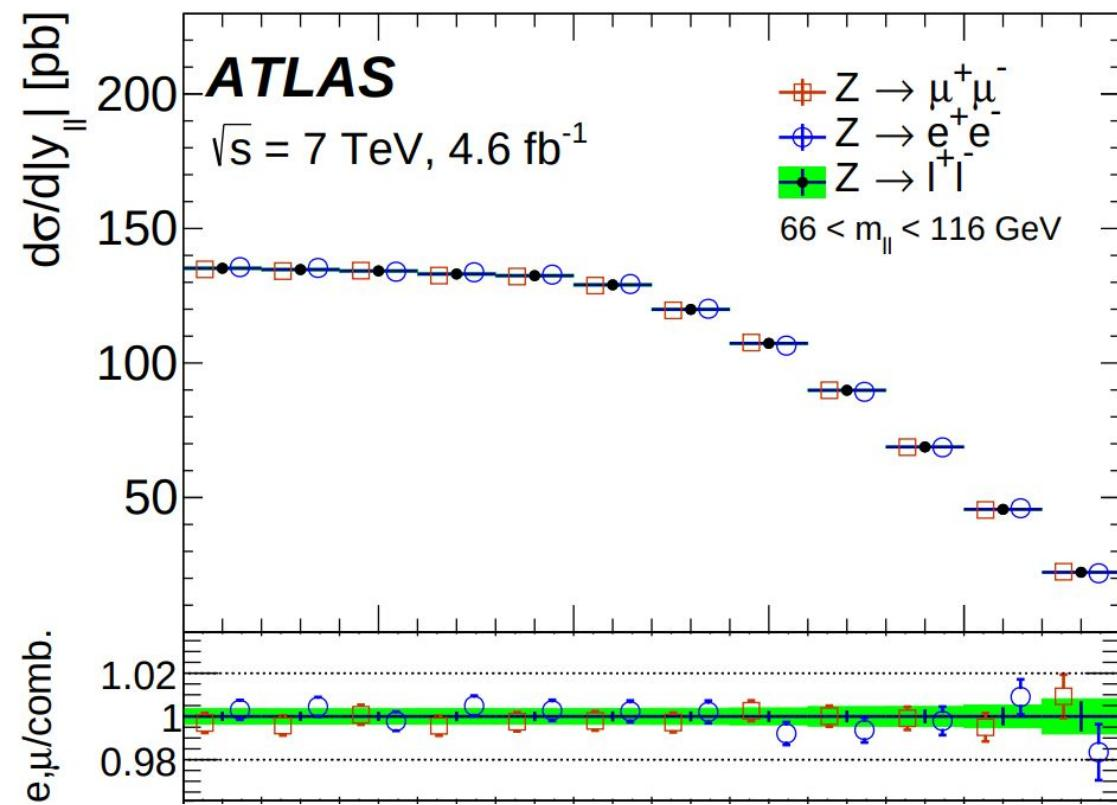
An example of detector cross-calibration: differential measurement of  $Z \rightarrow ll$  at the LHC using electron and muon final state.
