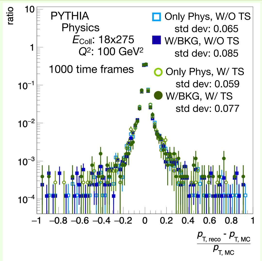
Good linearity between MC and reconstructed-track  $p_T$ . The  $p_T$  resolution of the time splitting is a little better than W/O time splitting.
