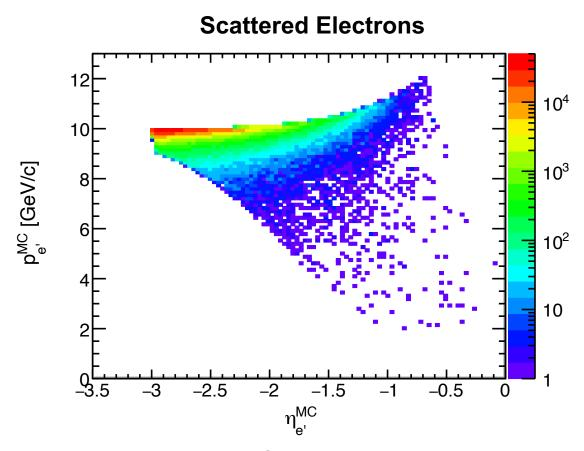
Relatively clean kinematics, with minimal overlap between all final-state particles. Scattered electron momentum remains very close to the incoming beam energy.
