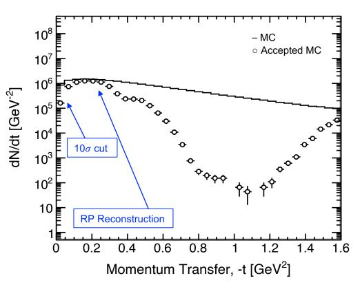
**Scattered protons** are mostly detected in the **Roman Pot**, not B0. Rather larger acceptance gap between B0 and Roman Pot for p' comparing to  $10 \times 100$  GeV<sup>2</sup>.
