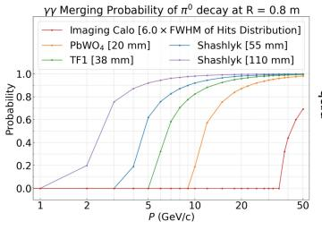
Upper limit of  $\gamma\gamma$  merging probability at  $\eta$  = 0, up to  $p_{\pi^0}$  ~ 35 GeV can be separable
