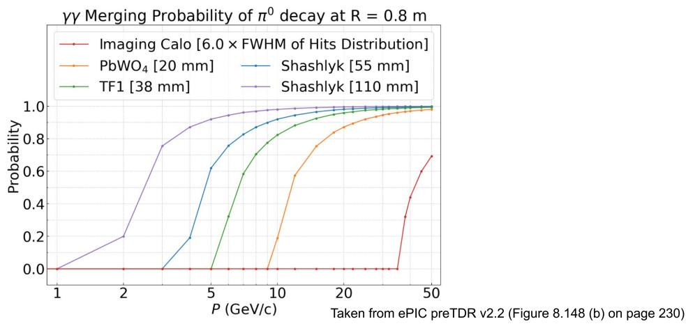
Upper limit of  $\gamma\gamma$  merging probability at  $\eta=0$ , up to  $p_{\pi^0}\sim 35$  GeV can be separable
