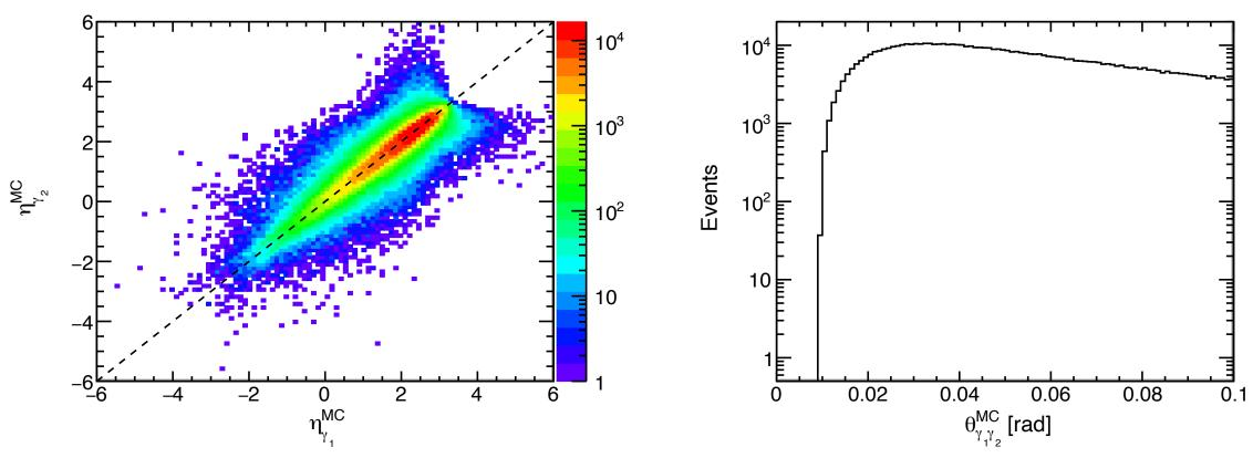
$\gamma\gamma$  are concentrated **within similar pseudo-rapidity** and threshold of  $\theta_{\gamma\gamma}$  is around 0.01 rad Very few events where we simply lose a photon by geometric acceptance
