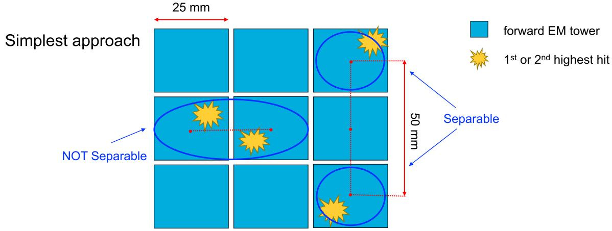
If distance between two highest hits is at least twice tower size (50 mm) to be separable
