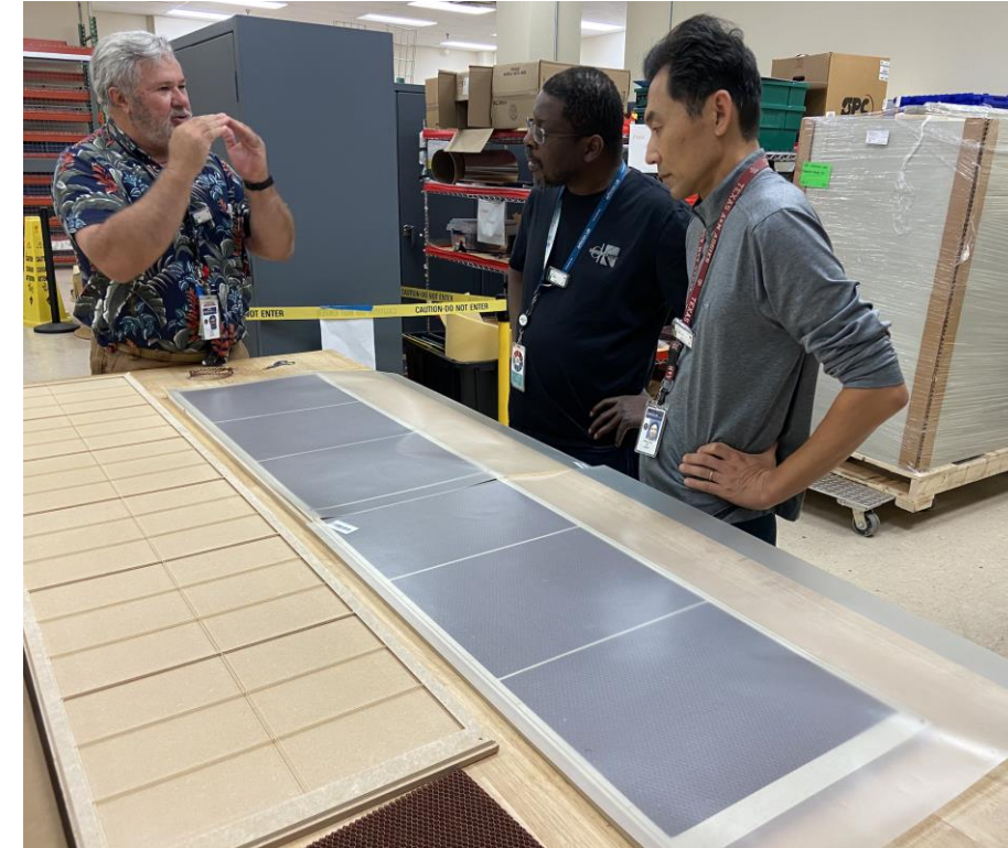
Sandwich the honeycomb b/w G10 skins
