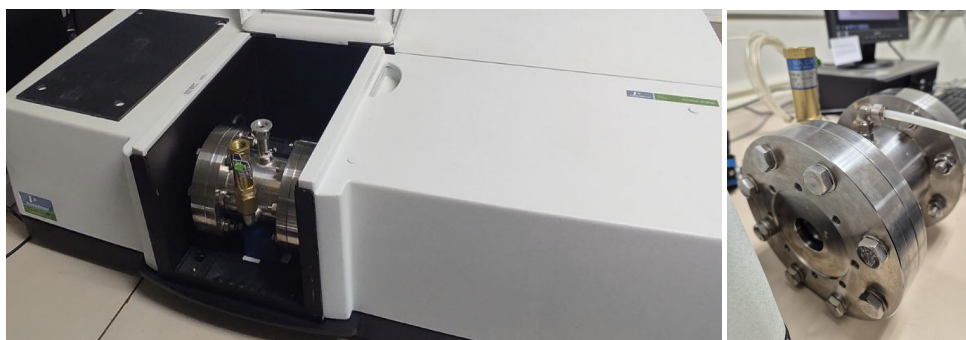
Figure 2: Setup for the monitoring of the C_2F_6 transparency in the 200-900 nm wavelength range.
