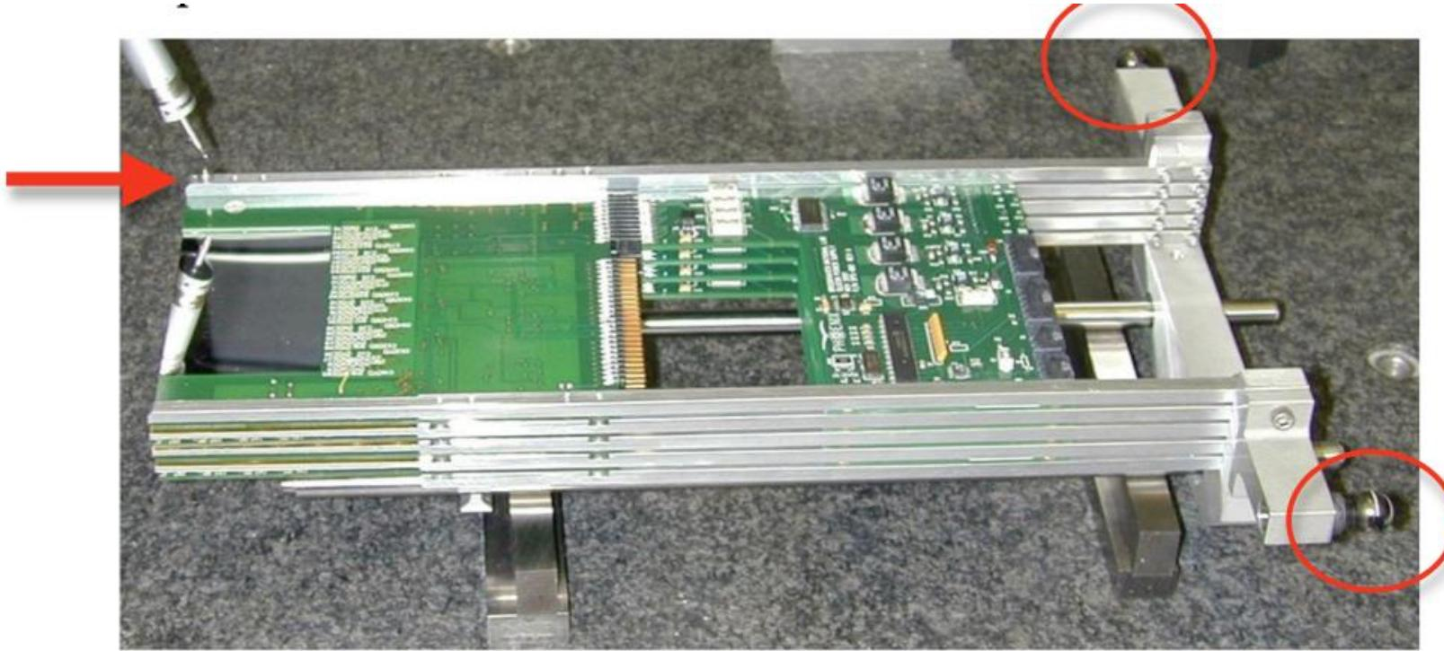
A detector package being surveyed in the lab (tabletop setup); Centering pin and reference point or point (0,0) on the detector package shown by arrow (top-left corner); Two tooling balls shown by circles (top and bottom right corners). Those tooling balls are the external reference used for the survey in the tunnel.
