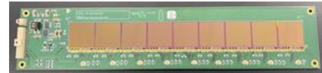
AstroPix Module 9 AstroPix sensors daisy-chained together on PCB.
