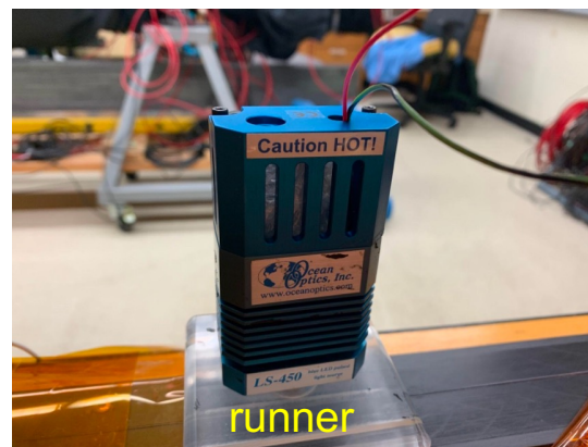
LED 370 nm; slides on acrylic runner
