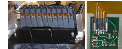
Fig. 3. Left panel: one end of a prototype BCAL module, showing two of its four columns of light guides. The LED pulsers are mounted on the side of the light guides attached to a common flexible cable. The free end of the flexible cable connects to the control board (not shown here). Right panel: BCAL LED pulser
