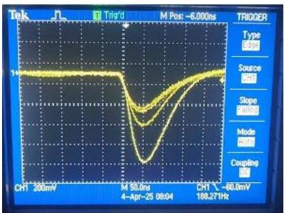
Sample signals from 16:1 multiplexing of a S14161-3050HS-04 4x4 array with a LYSO scintillator
