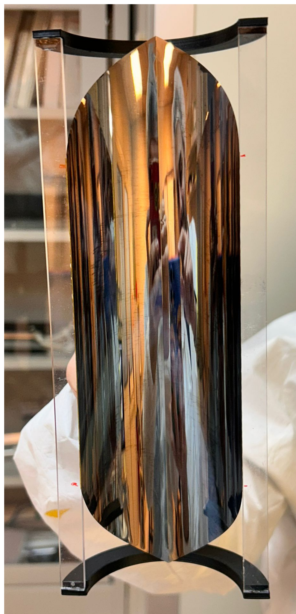
Two large size silicon pieces aligned, bent and kept in shape by local support structures
