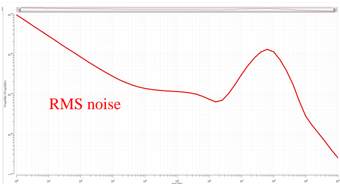
Figure 9. High pass active filter output voltage noise.
