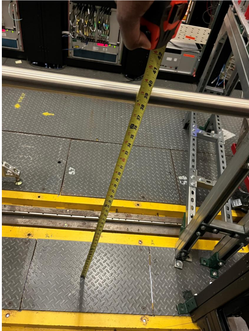
Beam pipe height: 39" (~99 cm)
