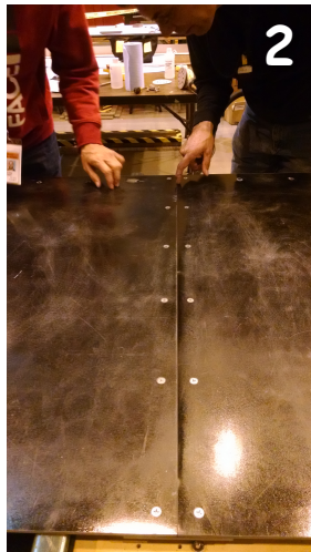
2 Drill and tap for joining panels
