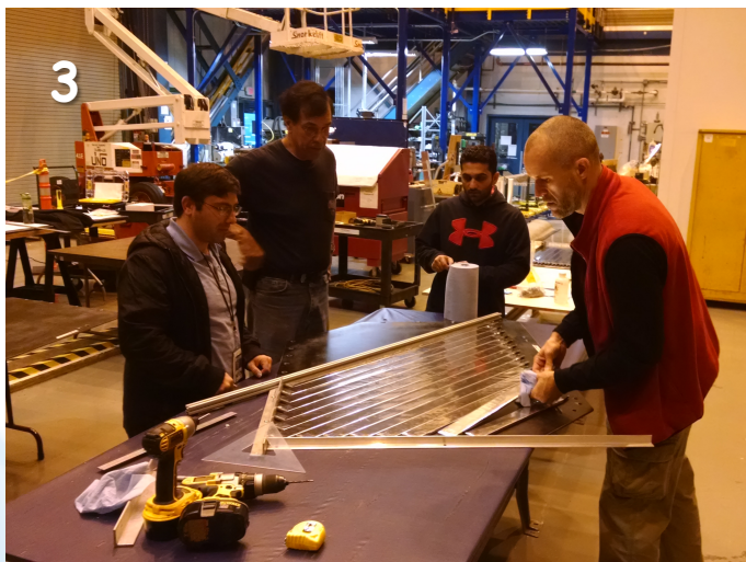
3 Glue on wrapped scintillators with light guides
