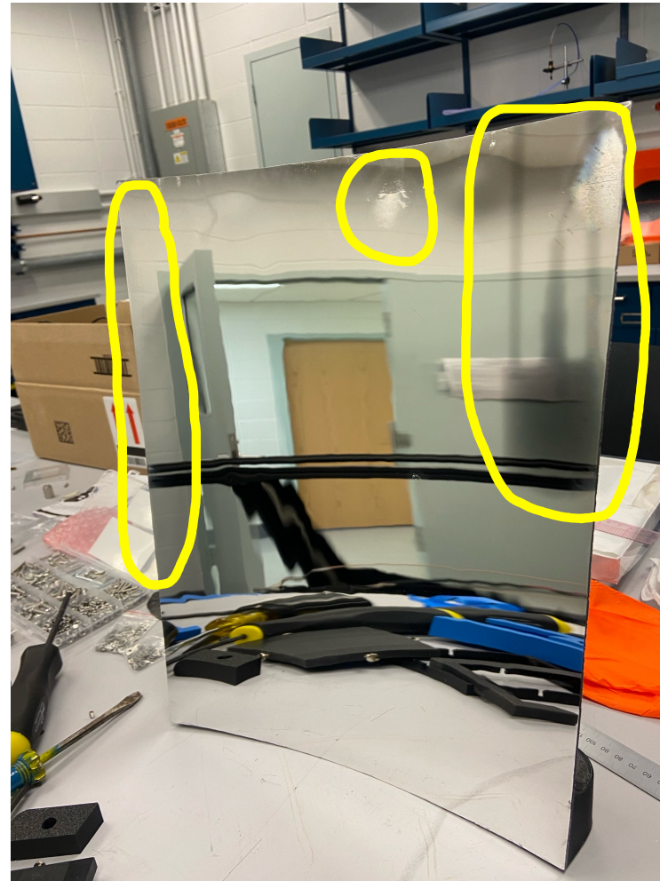
Gray area/Bad coating area
