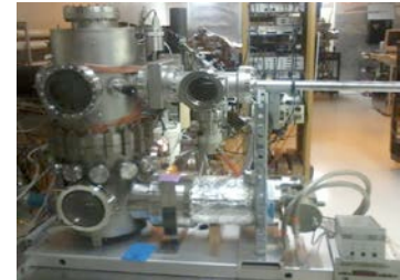
Evaporation deposition chamber for metallization
