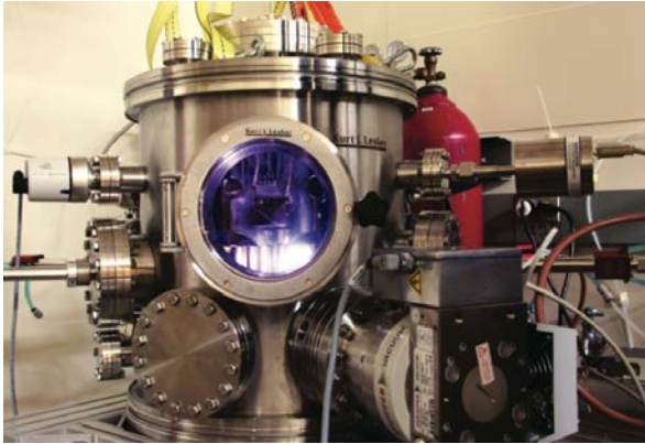
Off-axis RF Magnetron Sputter Deposition Chamber at Stony Brook
