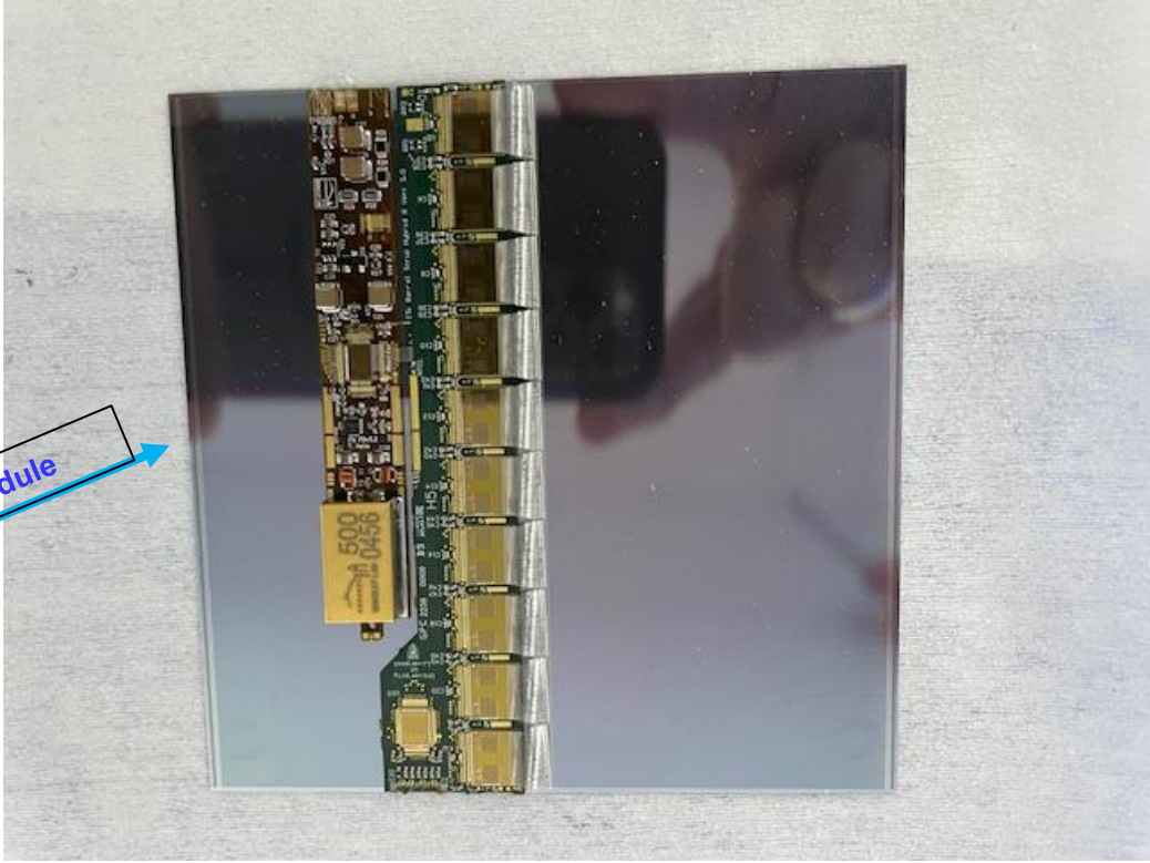
Silicon Module ready to be glued on the Bus Tap
