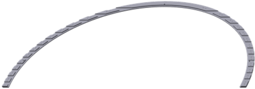
Back side of rim shaped to corrugation
