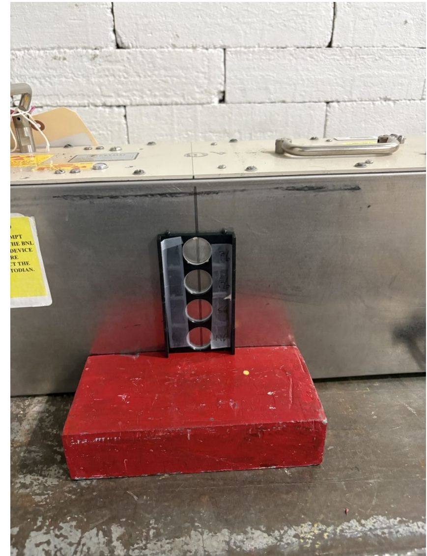
Samples during neutron irradiation
