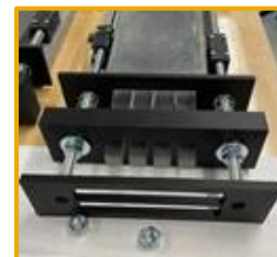
50cm-long SFIL at ANL (Scintillating Fiber Imaging Layer)
