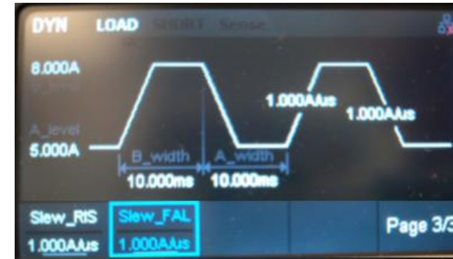
3A transient load response 60% to 100% ΔLoad
