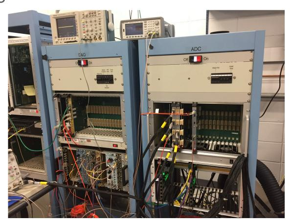
Test Stand in the Hcal Lab (cosmics tests, noise, pedestals, . . .)
