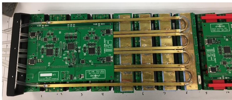
Test fit of Water Cooling on detector mockup
