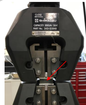
Epoxy bonding strength testing
