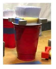
blocks made from mesh/fiber assemblies and tungsten powder cast with epoxy
