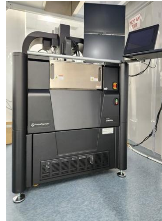
FormFactor CM300xi probe station in BNL's new shielded test lab
