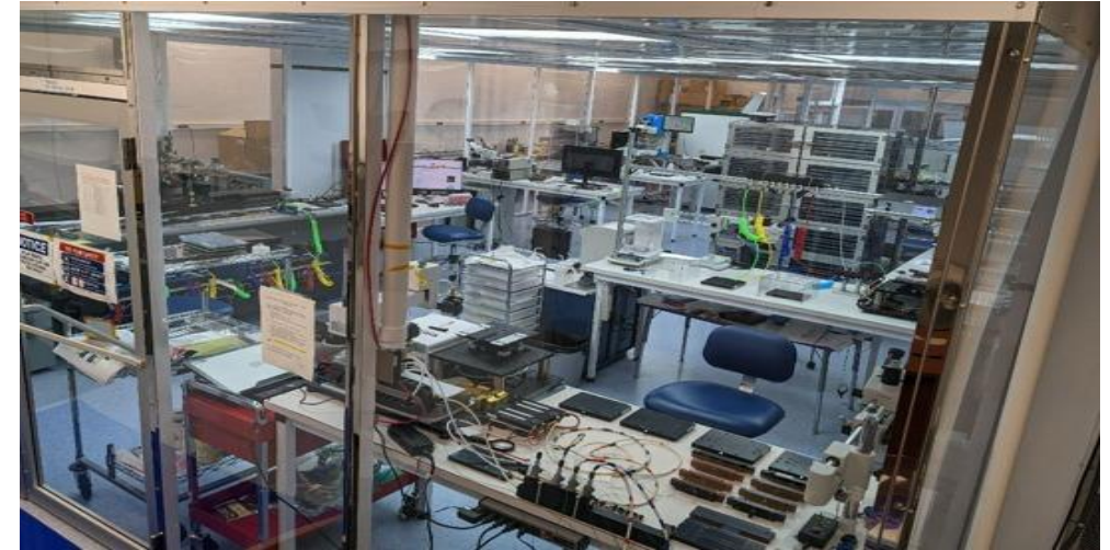
Assembly clean room (class 10,000)
