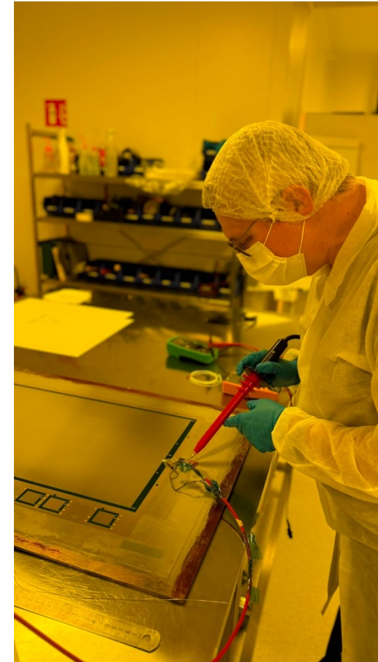
Bulk-micromegas mesh (HV Q/C)
