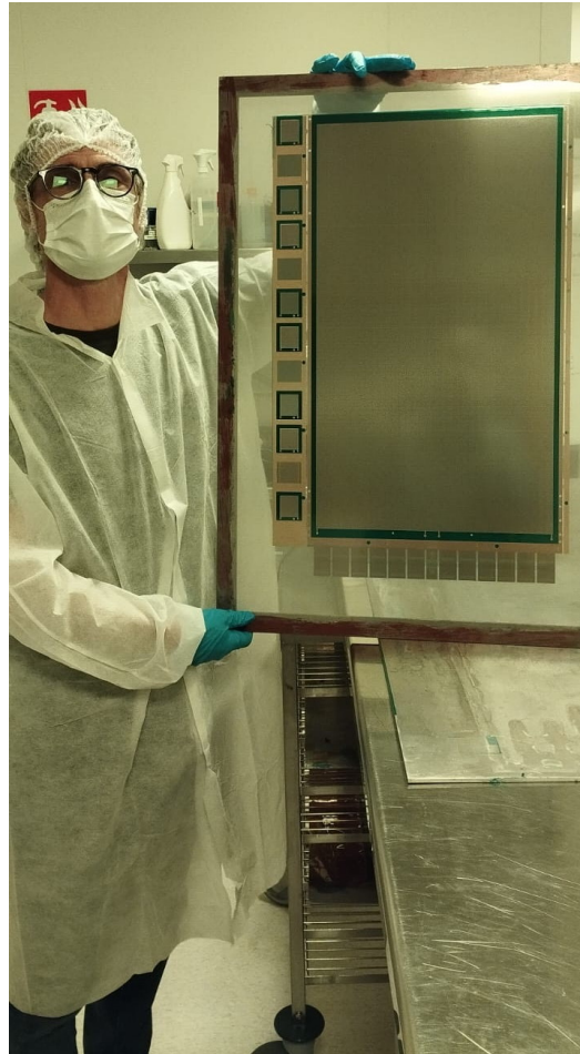
Bulk-micromegas mesh (before final cutout)
