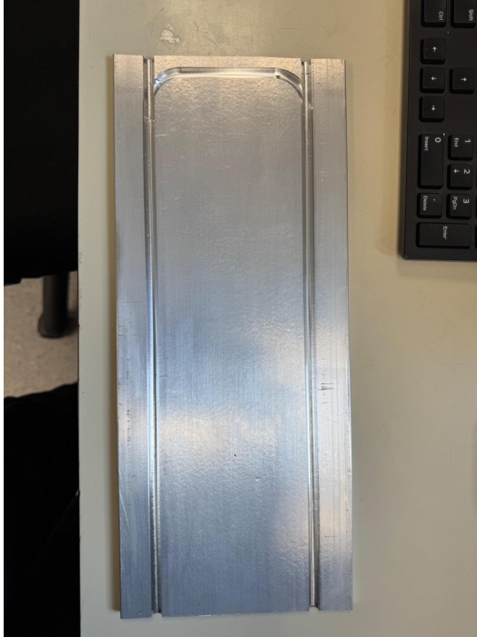
CNC-machined channel profile for copper pipe press-fit integration.
