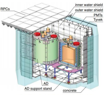
Double purpose: shield the ADs and veto cosmic ray muons
