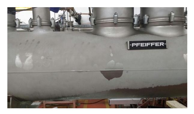
Leak in LN<sub>2</sub> shielding of cryostat (March 2017)
