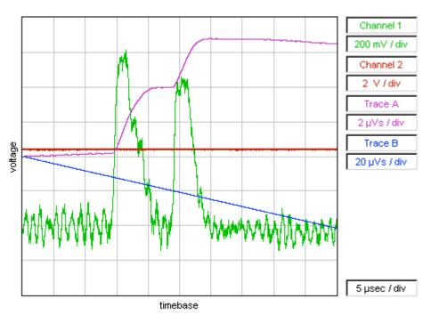
Au at the linac output, double pulsing trap electrodes to extract ions
