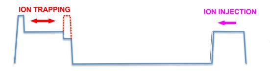
During injection and confinement the RHIC EBIS operates at ground potential.
