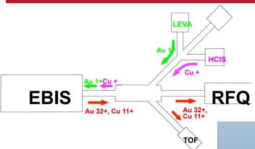
External ion injection provides most ion species (EBIS ~ a charge breeder)
