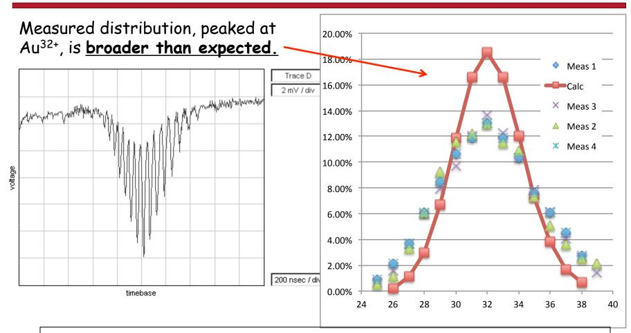
The proper distribution had been achieved on the Test EBIS. Need to work on ion injection to increase the intensity of Au<sup>1+</sup> in the electron beam, in order to improve the charge state distribution.
