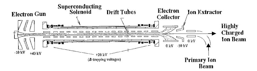
Radial trapping of ions by the space charge of the electron beam. Axial trapping by applied electrostatic potentials at ends of trap.
