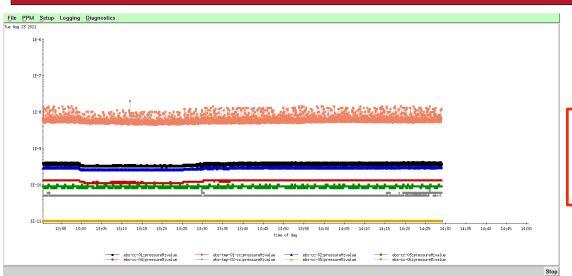
Pressure log for 7.6A e-beam with a 65ms ion confinement
