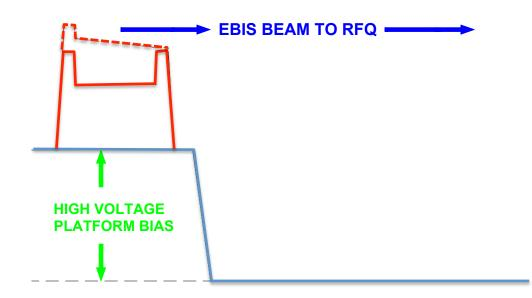
Just before ion extraction the EBIS Platform Voltage is applied such that the ions are extracted through 100kV (nominal) to attain the ~17keV/amu needed for acceleration by the RFQ
