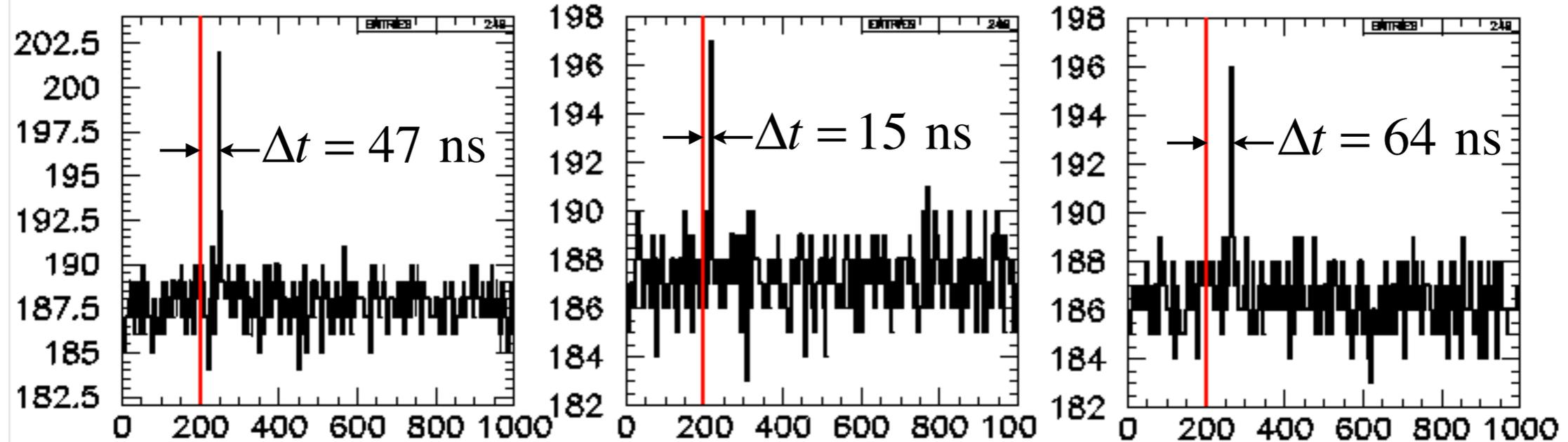
Two of the waveforms look like a regular signal, but delayed - could be due to fADC instability or another electronics problem
