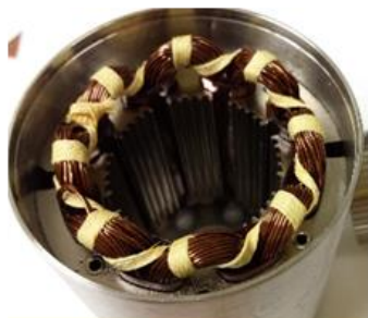
Radiation Hardness tests of the Electromechanical Actuator (up to 5 \cdot 10^8 Rad)
