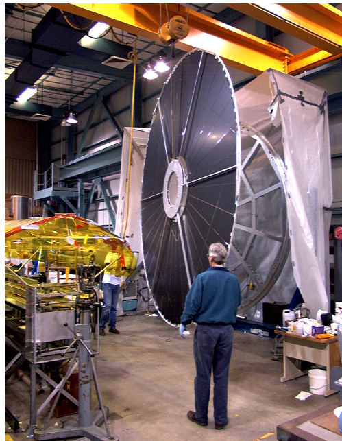
Figure 3.50: Photograph of the central membrane of the STAR TPC. The pattern of Aluminum strips is used to release electrons via laser flash as a calibration signal.
