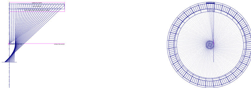
Figure 4.8: Drawings showing the projectivity of the EMCal blocks along the beam direction (left) and in \phi (right).
