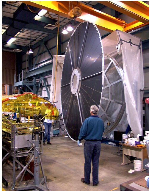
Figure 3.51: Photograph of the central membrane of the STAR TPC. The pattern of Aluminum strips is used to release electrons via laser flash as a calibration signal.
