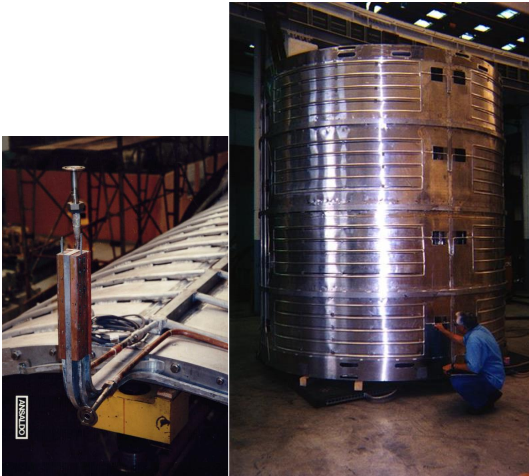
Figure A.8: (Left) Exiting leads — aluminum removed and niobium titanium soldered to heavy copper stabilizer leads (overlapping aluminum); (Right) Outer heat shield.
