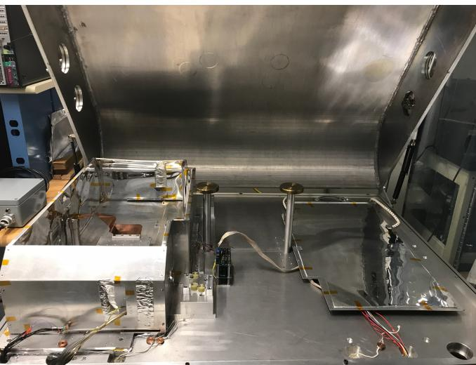
The test bed includes a 3 axis stage, a pair of integrating spheres to provide uniform Lambertian illumination, and optics to image a sub-pixel spot.
