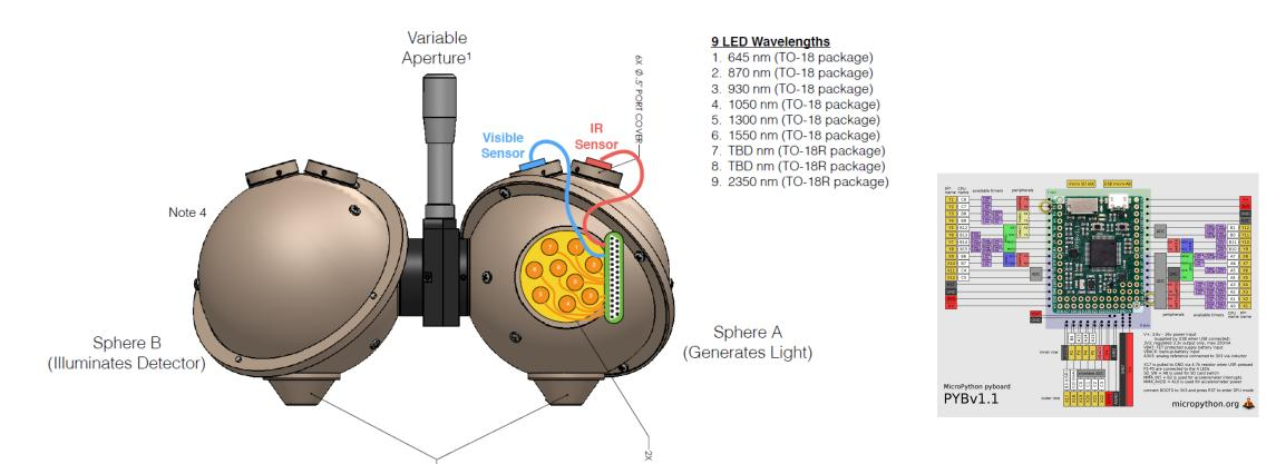
Figure 2 The internal chamber will house the detector on a 3 axis stage (left), a pair of integrating spheres to provide a uniform light source (Fig, 3), and additional optics to provide imaging of a sub-pixel spot on the detector plane or an image of the side port of the test dewar (not shown). Motor controllers (MCST 3601) integrated in the motor control box (right).
