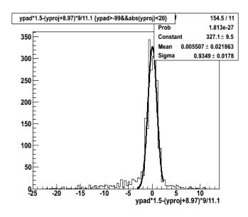
Example correlation between the y-axis of a 3 mm x 3 mm pad and the MWPC projection
