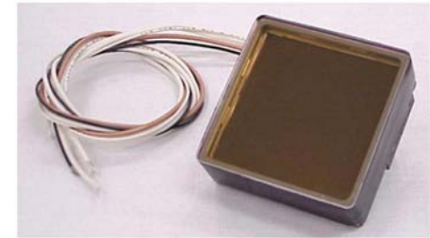
Photonis XP85112 64 channel, 10 \mu\text{m} pores
