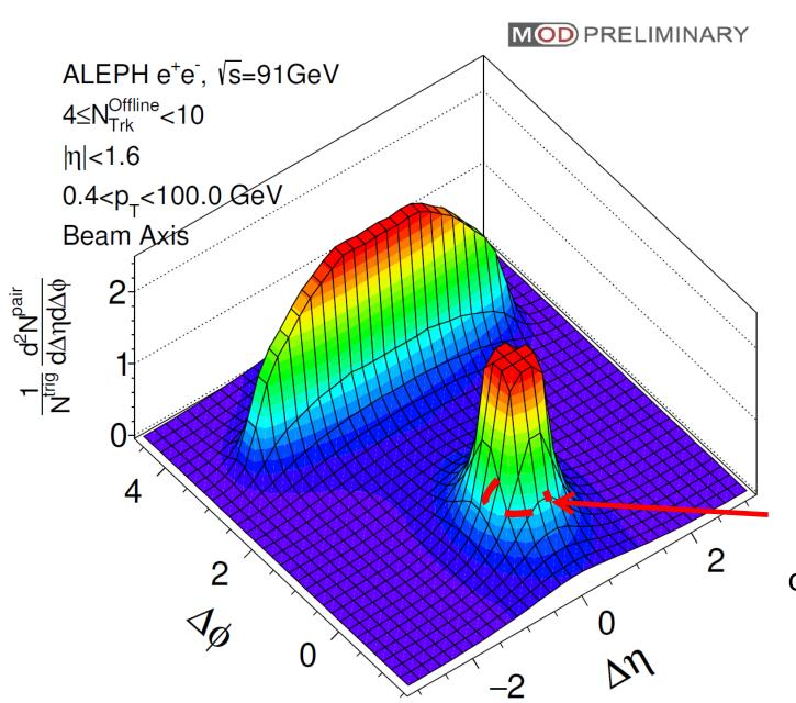
$$S(\Delta \eta, \Delta \phi) = \frac{1}{N_{trig}} \frac{d^2 N^{same}}{d\Delta \eta d\Delta \phi}$$
