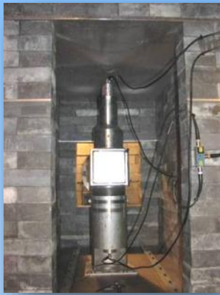
35 m Li-Glass Neutron Detector
