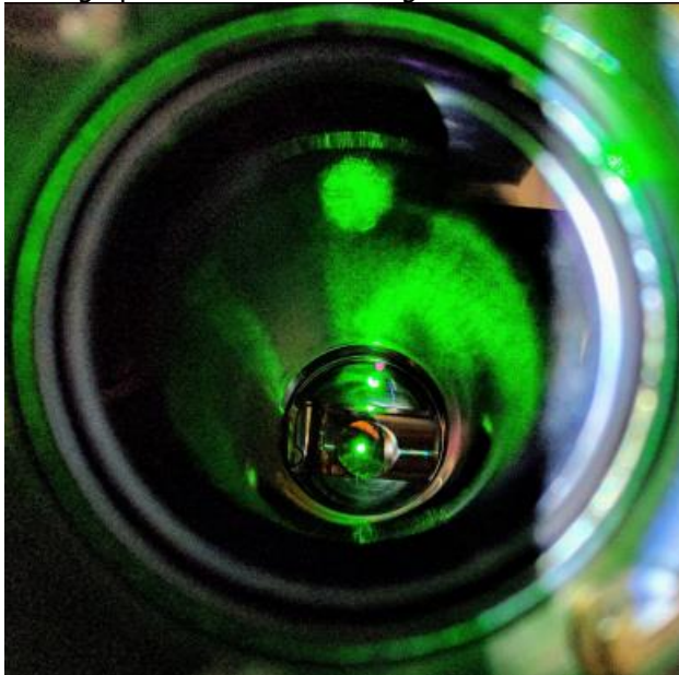
Photograph of fiber laser exiting vacuum chamber at location of laser exit window.
