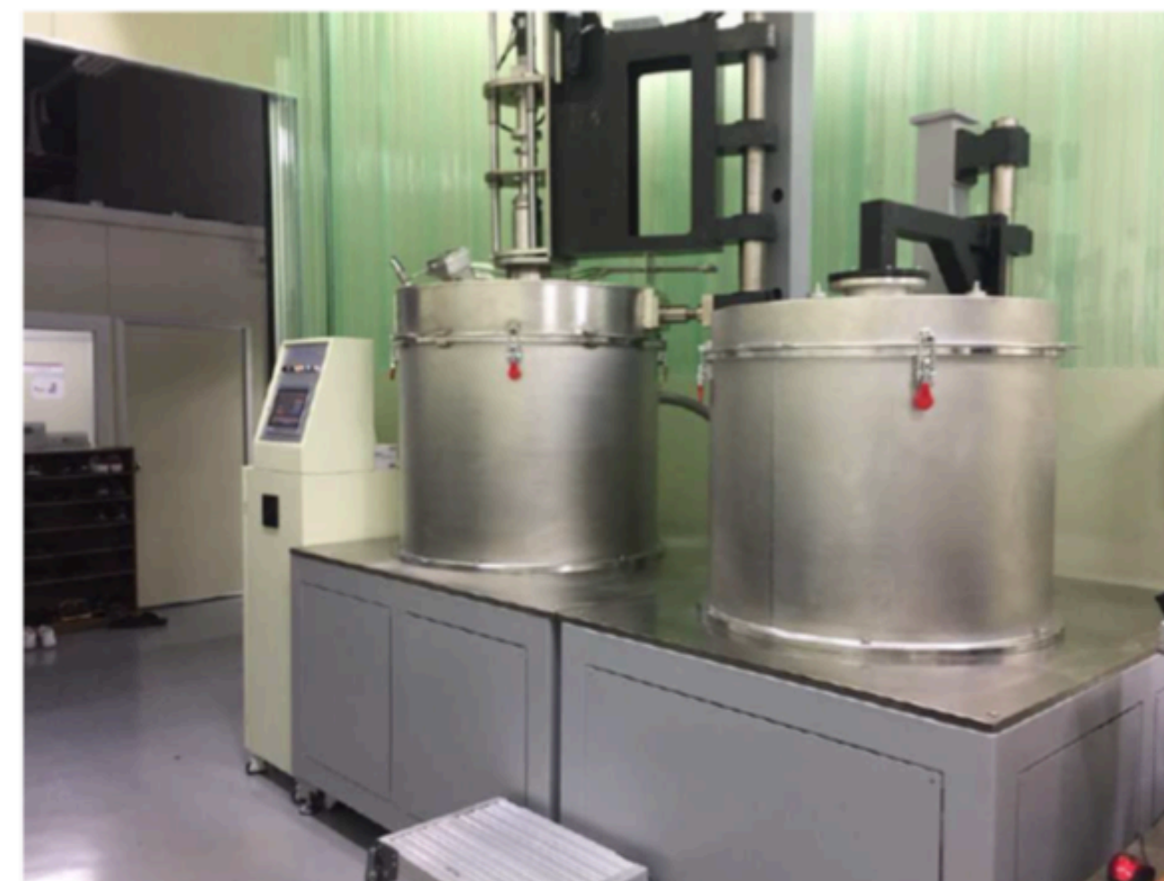
~ 100 kg NaI crystal (ingot) grower
