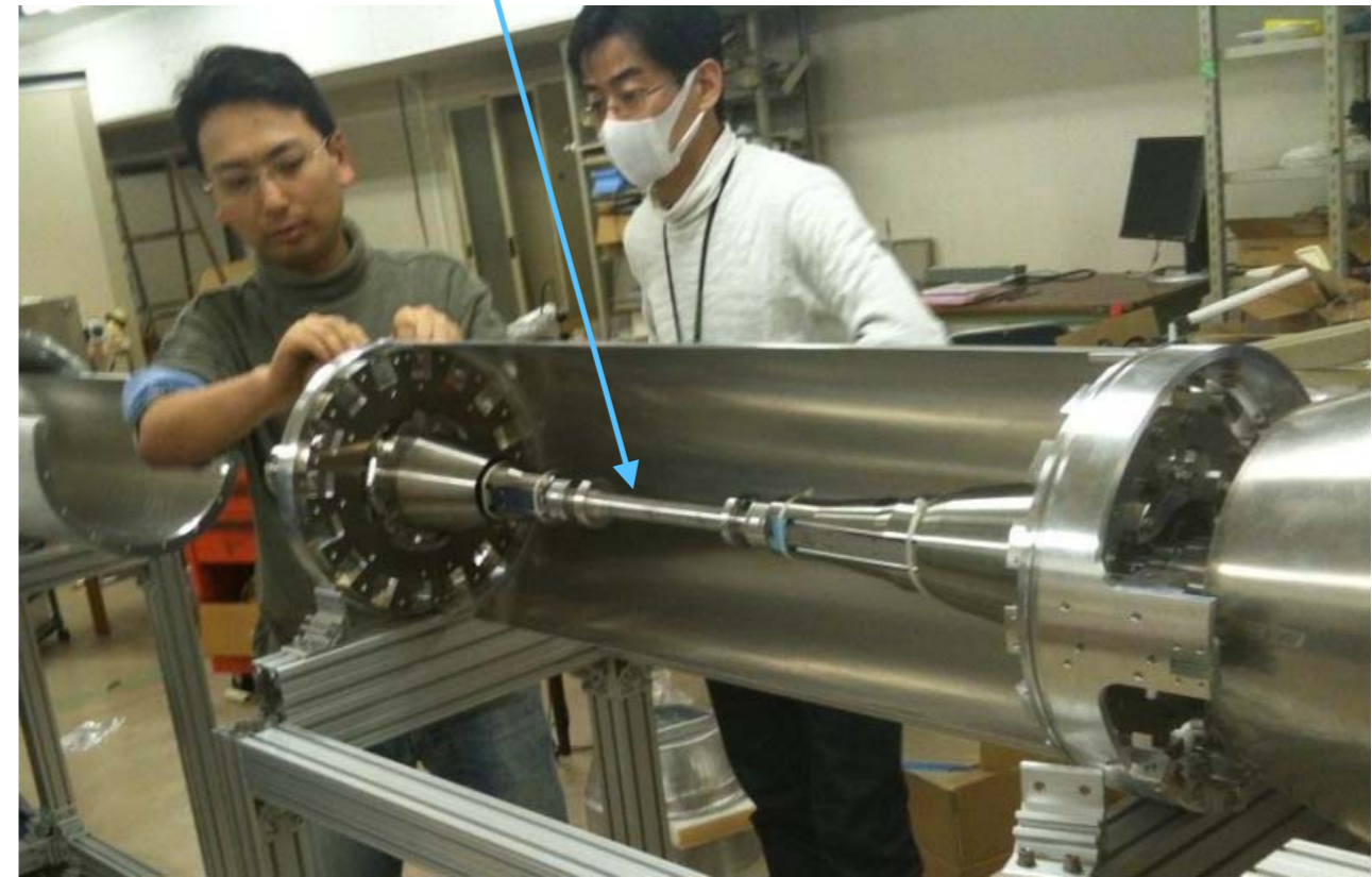
beryllium beam pipe at interaction point
