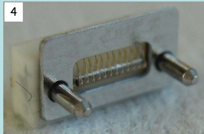
4 dust cover installed
