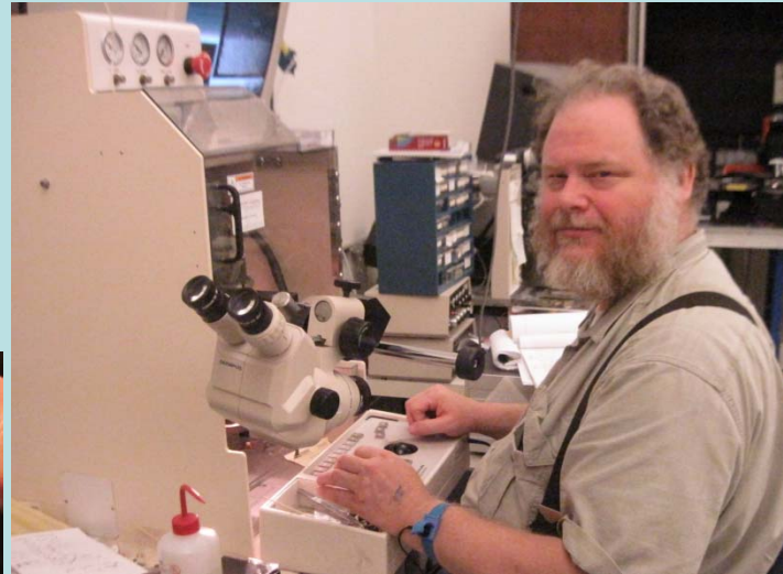
Wire bonding chips to board, board to opto-packs
