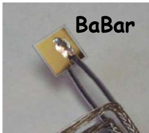
BaBar beam monitor: two pCVD diamonds 1 cm x 1 cm x 500 \mu m
