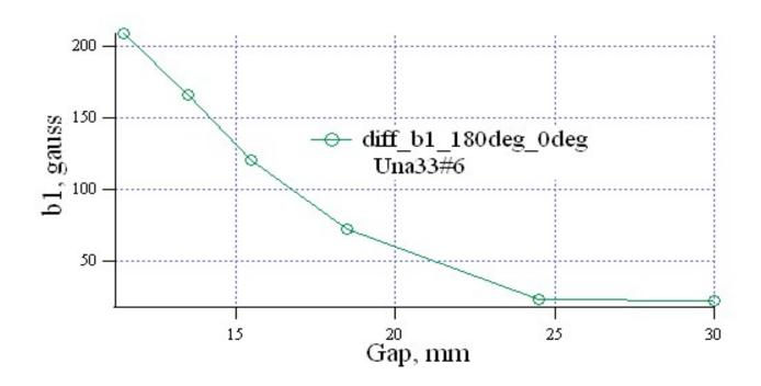
Difference of quadrupole component between rotated and non-rotated devices. Non-rotated device quadrupole component is compensated and has b1<50 Gauss for all gaps.
